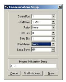
After modifying the EasySpan CommPort table above, the instrument's RS-232 settings must be modified to reflect the same settings. After matching up the settings [Click] on [Find Instrument] and the PC should find the instrument and display its model and serial number on the screen. If it doesn't, check the settings and cable to make sure they are correct.
